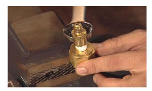
Take the Teflon Washer and place inside of the large threads of the CGA-320 adapter.
