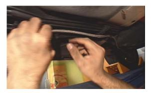
Take the 1/8" NPT Male to -4AN Male fitting and apply thread sealant to the NPT side of the fitting. Thread the fitting into the marked 'IN' side of the CryO2 Solenoid using a 3/8" wrench to tighten the fitting.
