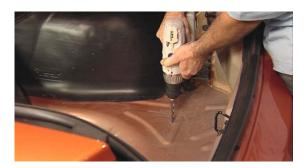
Replace the interior of the trunk and poke holes where the bolts can go through for mounting. Install the tank and mounting brackets with 5/16" bolts. You must have a 5/16" nut on the underside of the vehicle.
