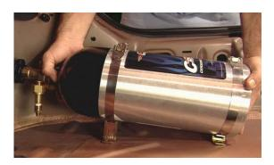
Remove the tank from the location, and using a 5/16" drill bit, drill holes where the Sharpie markings are. Also be sure to drill a hole where the stainless steel line can go through the trunk under the car. There should be a rubber grommet placed in this drilled hole for the line so that the sharp edges of the drilled hole do not puncture the stainless steel braided line under pressure.
